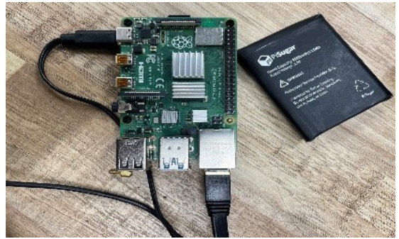
Fig. 3. The experiment system using a Raspberry Pi powered by a mobile battery
